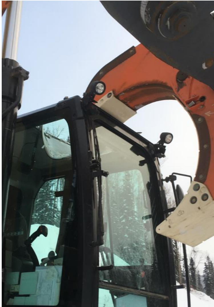
The pipe arm impacted the cab
