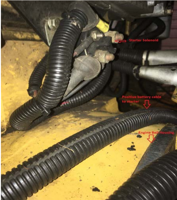
Battery cable location in relation to the engine bellhousing
