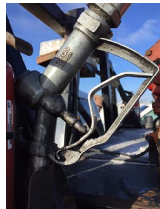
Correct Nozzle Placement
