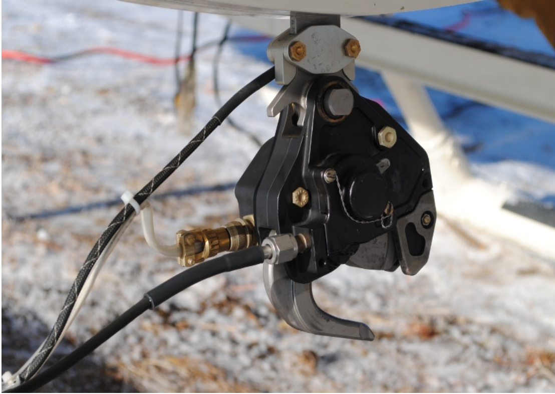
Photo showing normal hook configuration - new cable part installed
